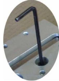
**3/** - Put **lock wire** in the threading of slider
