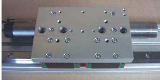
Torque the 4 screws of the coupling sleeves to 2.5 Nm
