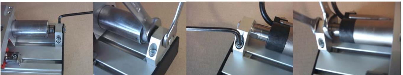
Check by moving back and forth several times that the module does not bind over the entire stroke and that **the slider does not rub**.
